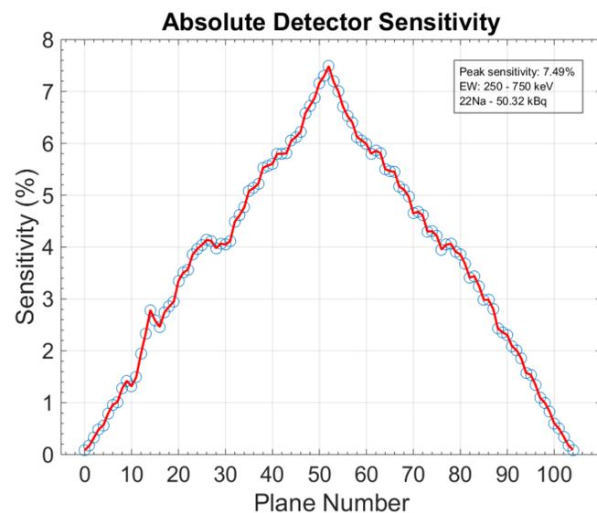
Figure 3: Measurement of absolute detector sensitivity yielding a peak sensitivity value of 7.49% compared to the vendor published value of 5.8%<sup>2</sup>.
