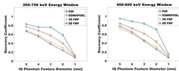
Figure 4: Recovery coefficients at energy windows of 250-750 keV and 450-600 keV for four different reconstruction methods: PSF, OSMAPOSL, 3D FBP and 2D FBP.
