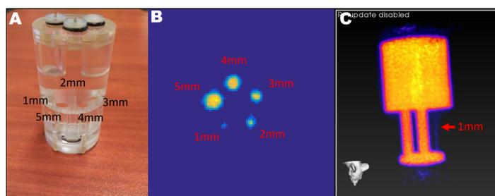
Figure 2: The NEMA NU 4-2008 IQ phantom demonstrating system resolvability down to 1mm.
