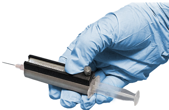
Figure 5. Shielded syringes can be utilized in the MR imaging room so that animals can be dosed as part of a dynamic imaging session.
